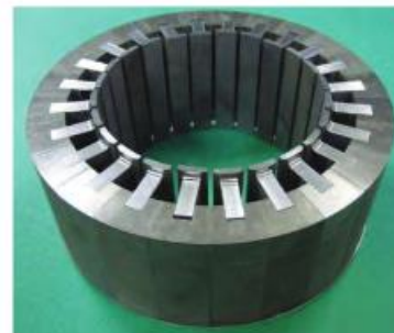
Composite stator of an induction motor made from SMC
